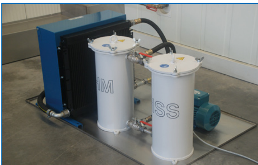
External coolant fine-filtration system with chiller
