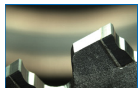
Example carbide tooth of a thin kerf saw blade (disposable saw)
